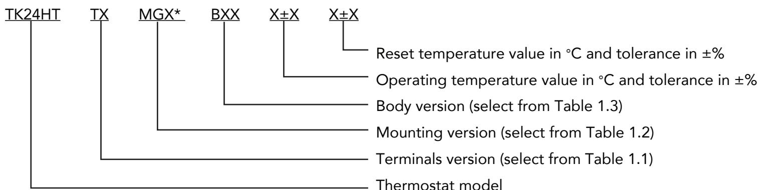
\*For screw cap mountings, screw parameters must be specified when placing an order.
