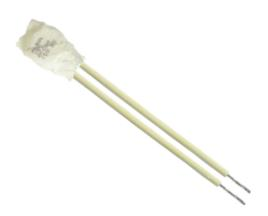
This resetable thermal cutout available from Calco Electric offers a small sized thermal cut out used for thermal protection of electric motors and transformers and is mounted directly into windings. Other applications include protection of heaters and controllers. The minimum current of protected circuit is 100 mA, the maximum current is set according to specifications. For any questions or to order, please contact Calco Electric.
